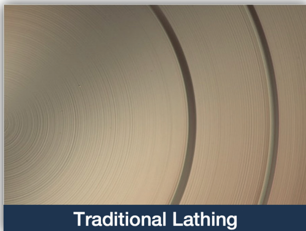
Figure 1. Traditional lathing relies on echelettes that are difficult to tumble polish due to their steep curves. High-resolution lathing creates echelettes that are essentially polished, which reduces light scatter.
