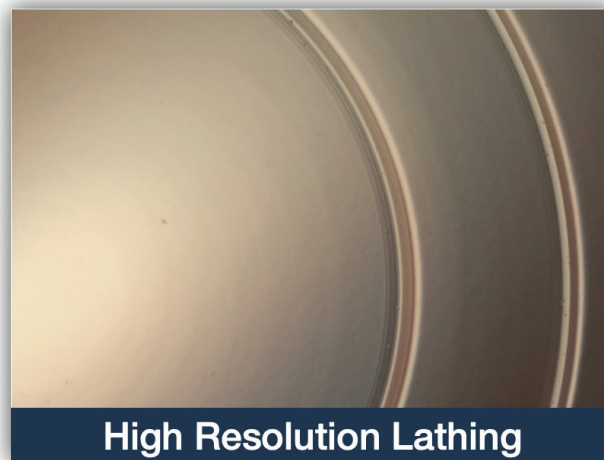
Figure 1. Traditional lathing relies on echelettes that are difficult to tumble polish due to their steep curves. High-resolution lathing creates echelettes that are essentially polished, which reduces light scatter.
